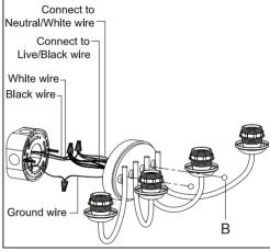
Step2:Wire fixture to wires in outlet box. Copper wire is for Ground. Attach canopy to mounting bracket and tighten with ball nuts。
