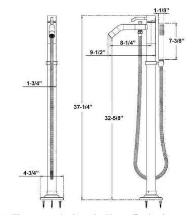
Use on concrete floors requires special installation. We recommend using a plumbing proffessional.
