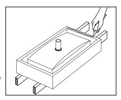
6 Mounting holes are provided on the rear of the lavatory so it can be secured to the wall if desired.
