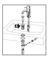
Mount the faucet and drain assembly (not included) on the sink following the manufacturer's instructions. Be certain to apply a bead of sealing putty on the underside of the drain (Part "A") in order to ensure a watertight seal between the sink and drain. Remove excess putty after installing drain on sink.
