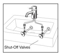
Connect supply line to faucet (finger tight) and carefully bend tubes to engage with the supply shut-off valves. Tighten connections at faucet and shut-off valves for secure seal.
