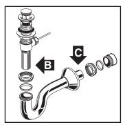
Connect trap to drain assembly hand tight to check alignment. It may be necessary to cut off part of the tailpiece (area "B") or part of the horizontal leg of the trap (area "C"). Secure joints for watertight assembly.
